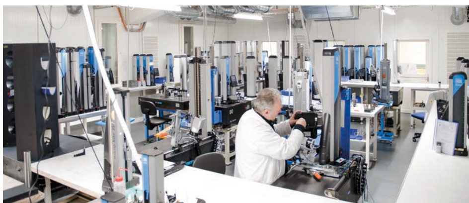
Calibration laboratory for TESA height gauges
